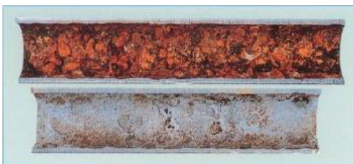
0.5 mm-thick scales can increase power consumption to 160%
