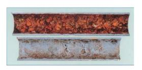
0.5 mm-thick scales can increase power consumption to 160%
